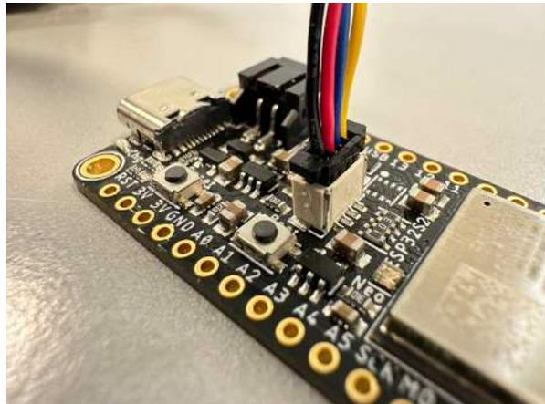
3.31 Qwiic connector on an ESP32 Feather
