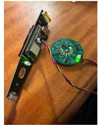
Controller PCB being tested with Scanner PCB
