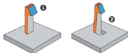
3.22 Undercut from snap-fit and possible solution
