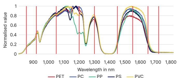
Figure 2.5: Spectroscopy plot, with PlasticScanner wavelengths (red lines).
