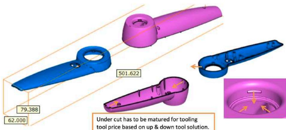
3.40 Mould layout sketch from manufacturer, with markings of mould insert and pull-out direction
