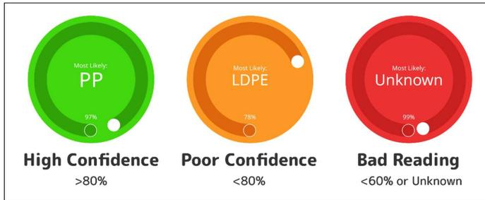
Figure 11: The LCD output based on the ML models prediction.
