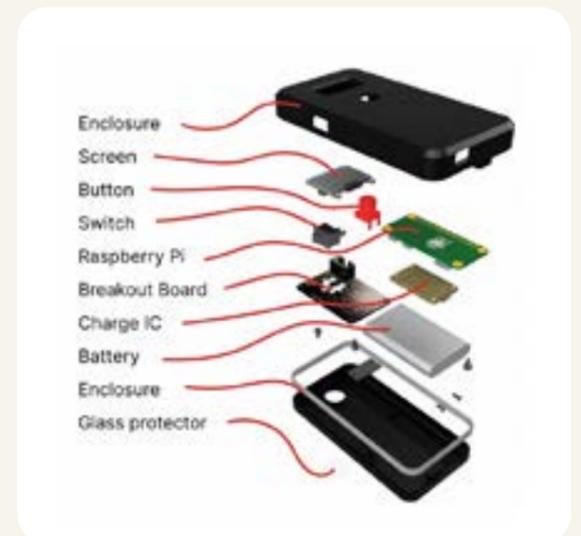
Figure 3: Exploded view of Jerry's prototype
