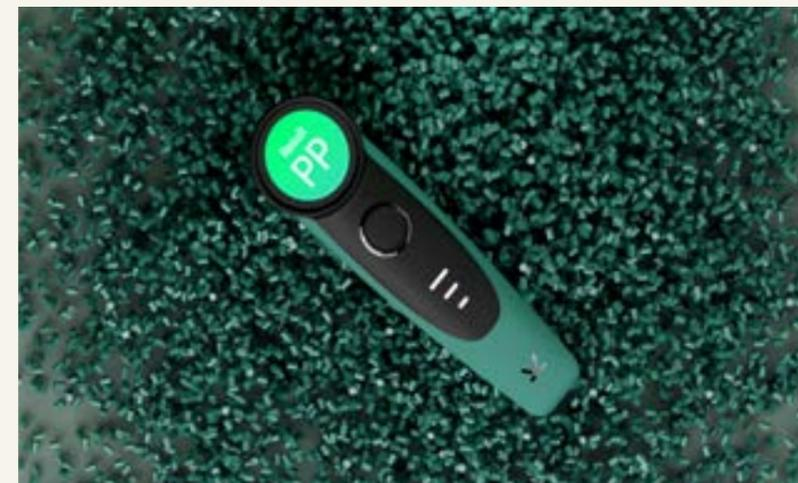
Figure 69: Plastic scanner on granulates from recycled PP
