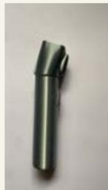
Figure 38: Model 5 - Oval handle 10 degrees angle
