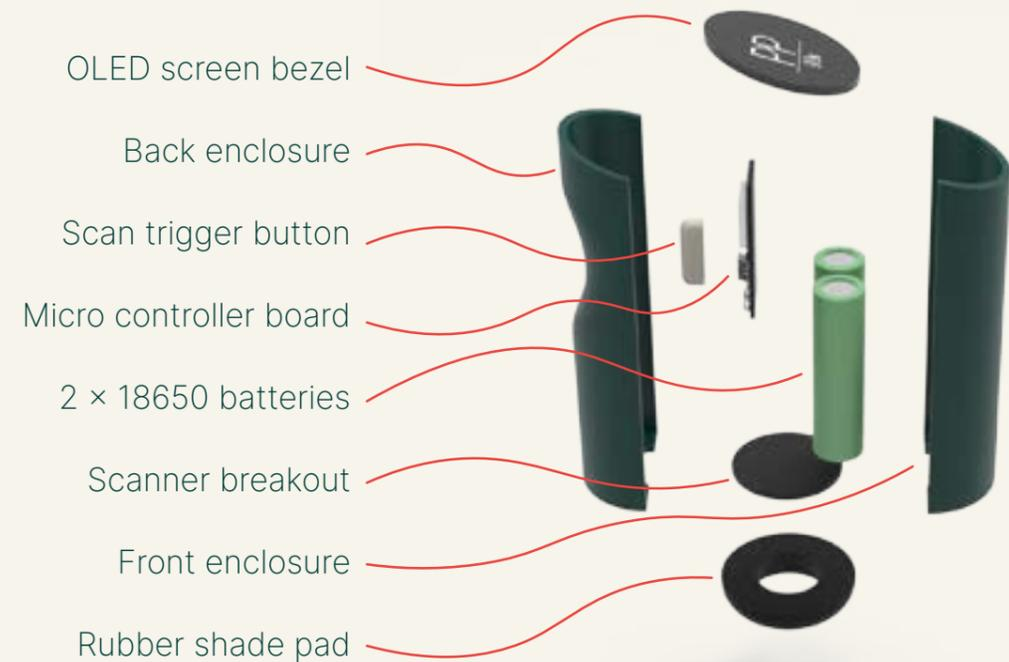
Figure 22: Exploded view of Q3 concept
