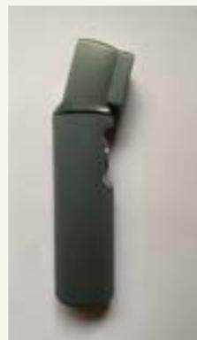
Figure 36: Model 3 - Cylindrical handle 10 degrees angle
