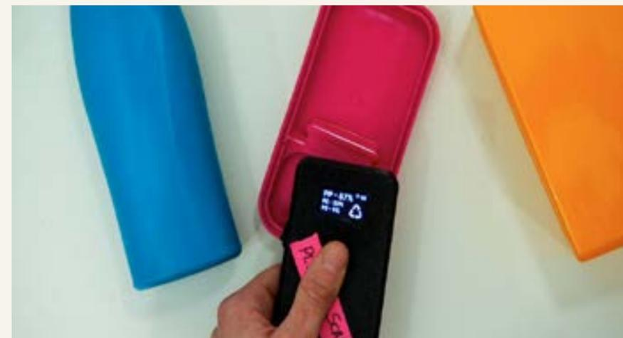
Figure 2: Plastic scanner scanning plastic product
